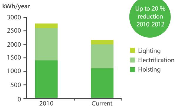
The calculation is based on an elevator speed of 1.6 m/s, a load of 1000 kg, 200,000 starts/year, a travel height of 45 m and 15 floors
